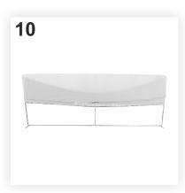
9. Add the second horizontal bar with previously mounted corner elements at the top of the system thus formed so that you'll get a complete frame. Now the PopUp structure is ready. 10. To add the textile graphic, you need to undo its zipper or velcro band, as the case may be. Then insert the graphic on the PopUp structure through the top, as in the adjacent picture.
